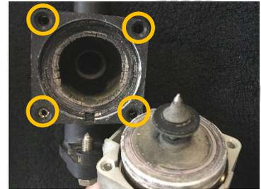
**3.** Take off the upper part of the housing including the coil and remove the old seal. Check the coil for corrosion. Replace if necessary.
